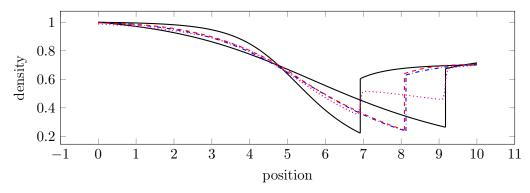
Comparison of the HDM,  $L^2$  projection (without snapshot alignment), and ROM-IFT on a nozzle flow problem with two training parameters. Legend: training snapshots (——), HDM solution at test parameter (----),  $L^2$  projection of test parameter onto reduced basis (······), and ROM-IFT solution at test parameter (----).
